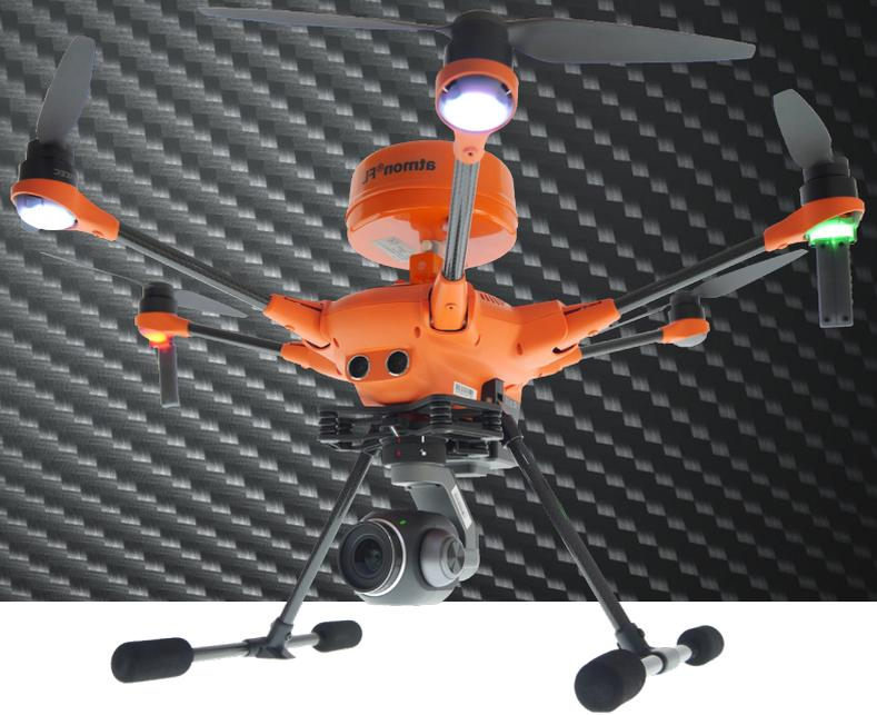
The Atmon FL for the H520 and H520E is one of the lightest mobile air analyzer on the market. It can fly on smaller drones, making it much easier to perform measurements, transport, and reduce the cost of a flying platform.
